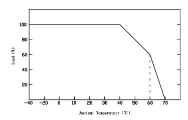
• Load carried in accordance with the load derating curve, according to the ambient temperature derating, in order to extend the running life.
