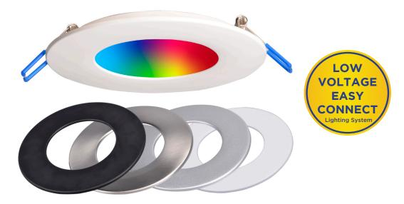
Lovo™Slim 12-in-1 is the first RGB LED recessed light that gives you the ability to customize on the spot! At 8 Watts and 800 lumen output, each LovoSlim fixture allows you to choose between RGB colors and change the fixture finish color instantly with magnetically attached trim rings! With Prism designed low voltage FC cable system, you can daisy chain up to 6 fixtures in a row and if more lights are needed, simply add multipoint connectors to link all the lights to a single power supply.
